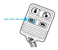
Pressing the trunk control will prevent the alarm from sounding until the trunk is closed again.
